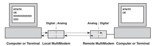
Figure C-2. Remote digital loopback test.
